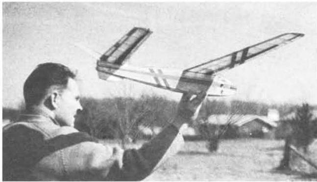
The author hand-launches his light-weight powered soarer. Built-up construction will please those who like the good feel of open framework, and the sun shining through the covering.
